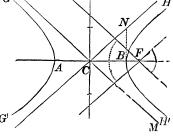
The cosine of the angle NCB formed by the asymptote with the transverse axis is equal to CB divided by CN; that is, to
